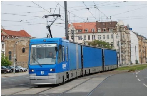
Fig. 2. Example of a three-section tram for urban freight (Hinčica, 2022)
