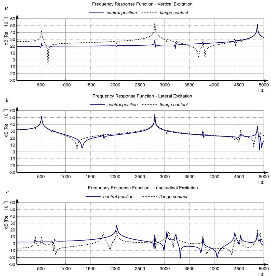
Fig. 6. Frequency Response Functions due to the vertical (Figure 6*a*), lateral (Figure 6*b*) and the longitudinal force (Figure 6*c*)
