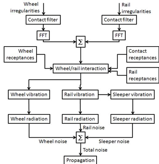
Fig. 1. TWINS model for rolling noise generation
