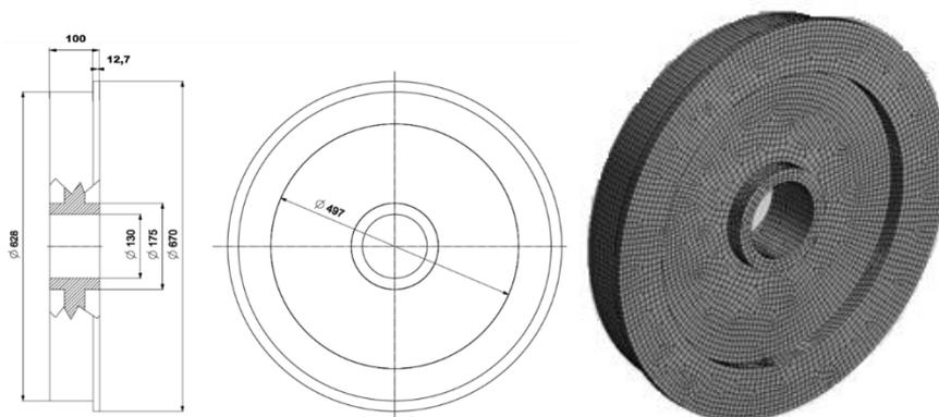
Fig. 4. Basic dimensions of wheel model and adopted mesh
