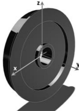
Fig. 3. Monobloc tram wheel and the associated reference frame (y – axis is perpendicular to the wheel plane)
