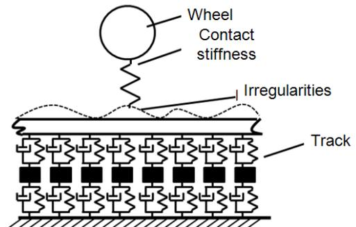
Fig. 2. Scheme of the wheel rail system excited by rolling surfaces roughness
