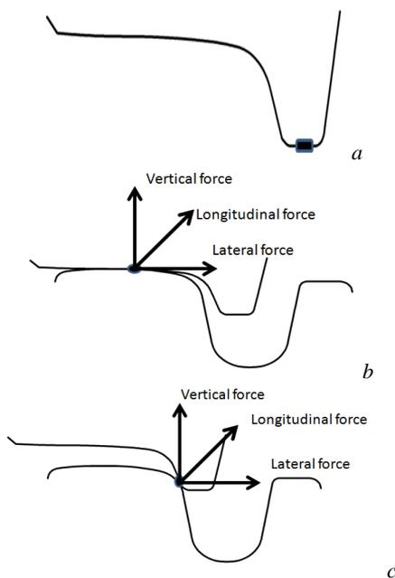
Fig. 5. *a* – point of Frequency Response Function study, *b* – contact point corresponding wheelset central position, *c* – flange contact point
